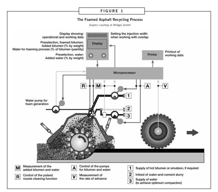
**Traffic.** Foamed asphalt can be compacted immediately, and can carry traffic almost immediately following compaction. Often the entire process from pulverizing and injecting to final rolling can be completed in 30 to 45 minutes.
